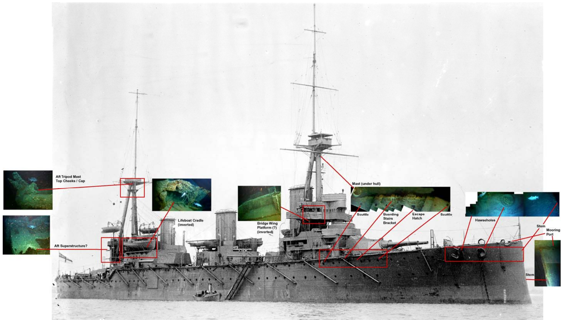
Features confirming the identity of HMAS Australia (Image: Heritage Branch after Royal Australian Navy/ Defence Maritime Services 2007 Survey)
