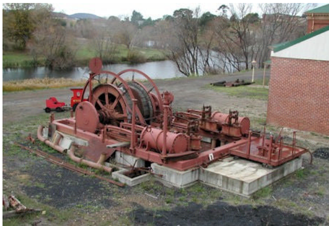
Hebburn steam winding plant, Goulburn, NSW. Originally from the Newcastle coalfields.
